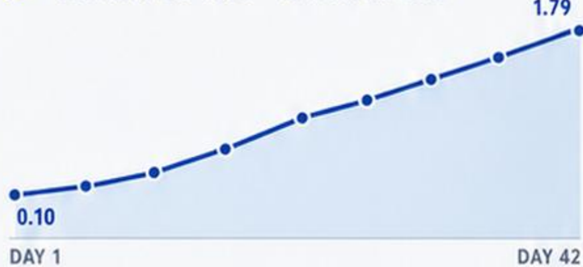
VENTILATION RAMP · M 3 /HR PER BIRD
